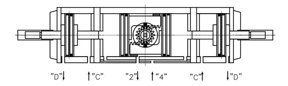
Fully Closed Position From chart 1 we can see that this position is obtained when air is supplied to port 4 and port 2 is in the
